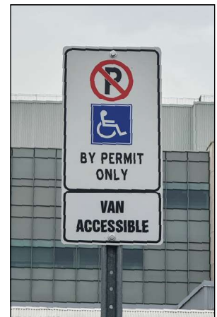
Example of Type A “VAN ACCESSIBLE” vertical signage.
