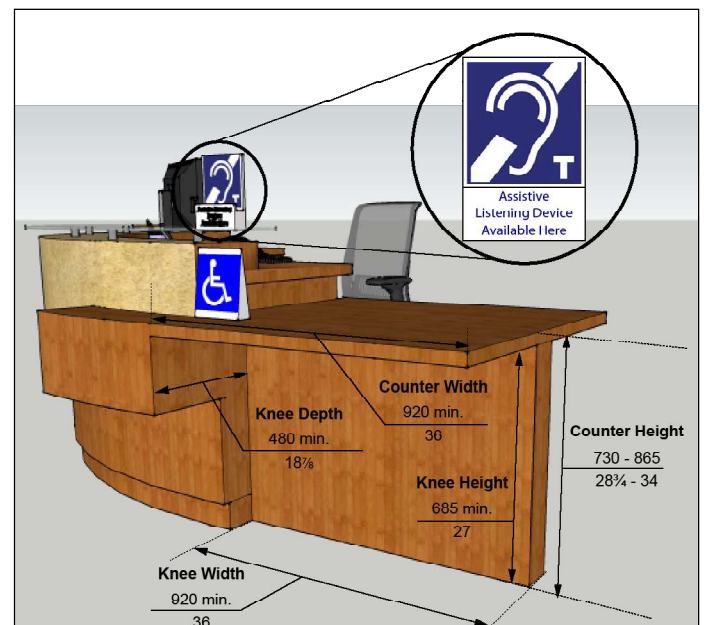
Figure 110: Dimensions of Accessible Service Counter
